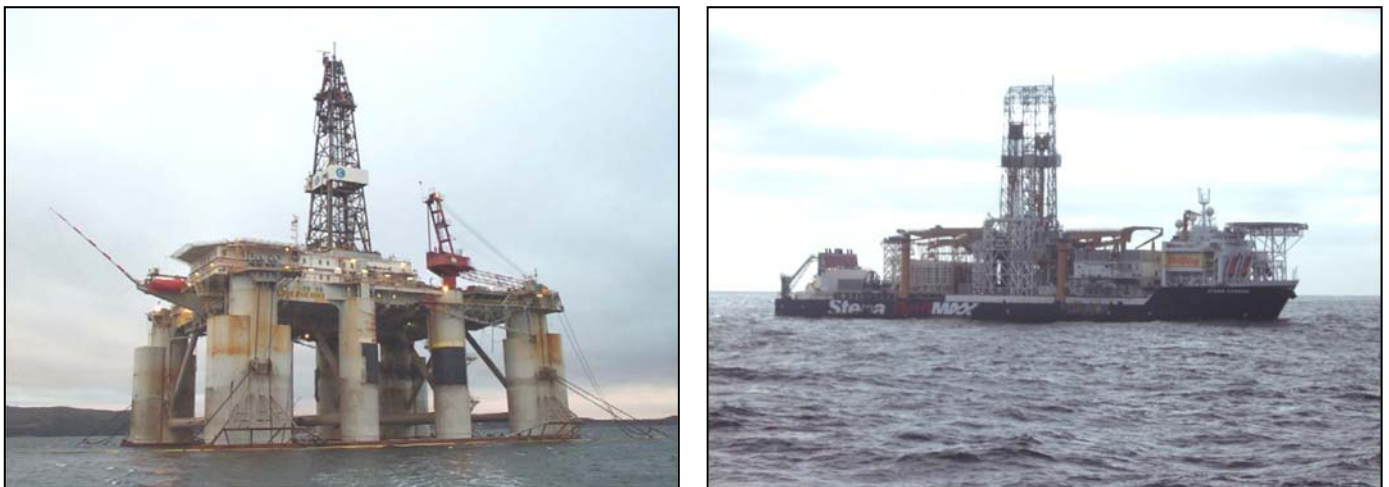
Figure 2.3: Typical Semisubmersible Drilling Unit (Left) and Drill Ship (Right) (Amec 2014)
